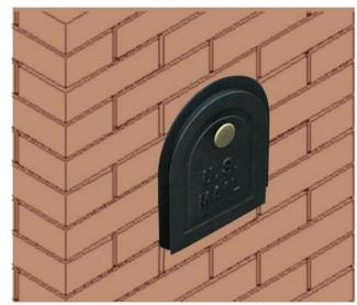
3. Apply a generous bead of clear silicone adhesive around the arch of your mailbox and insert you new door into the old mailbox frame. Push the door in until it is flush with the brick, stone, or stucco.
