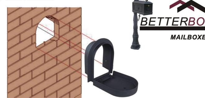
2. Check for proper fit and make final surface preparations.
