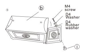
Open the door of the mailbox(b), then attach large brass knob(i) to the front of the door with M4 screw, D4 washer and D4 rubber washer.
