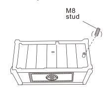
With the bottom facing up, insert M8 stud into the screw hole at the bottom rear of the mailbox.
