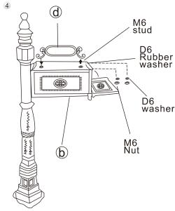
Place 2 D6 rubber washers over 2 M6 studs pre-inserted into the bottom of the number plate (d) . Secure the number plate (d) from inside the mailbox (b) using 2 D6 washers and 2 M6 nuts.
