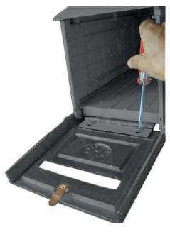
Step 2: Attach the new door to the hinge using the 2 screws from step #1 above. Do not fully tighten the screws at this time.
