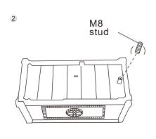
With the bottom facing up, insert M8 stud into the screw hole at the bottom rear of the mailbox.
