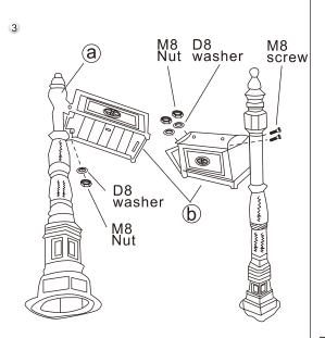
Attach the mailbox(b) to the post(a) on the bottom side with M8 nut and D8 washer and on the top side with 2 M8 screws, 2 M8 nuts and 2 D8 washers
