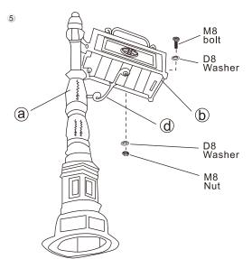
Attach the scroll (d) to the post(a) by placing the welded screw located on the scroll into the hole on the post. Secure the scroll to the mailbox(b) by inserting the M8 bolt and the D8 washer through the mailbox and the scroll from inside the mailbox. Place D8 washer and M8 nut over the bolt and tighten.
