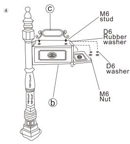
Place 2 D6 rubber washers over 2 M6 studs pre-inserted into the bottom of the number plate(c). Secure the number plate from inside the mailbox(b) using 2 D6 washers and 2 M6 nuts.
