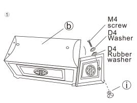
Open the door of the  $\mathsf{mailbox}(b)$ , then attach the large brass  $\mathsf{knob}(i)$  to the front of the door with M4 screw, D4 washer and D4 rubber washer.
